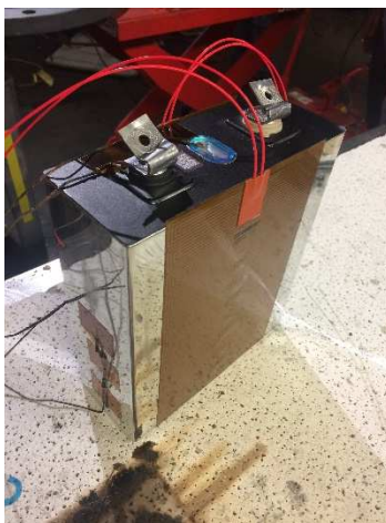
Figure 3 – Thermocouple and Heater setup
