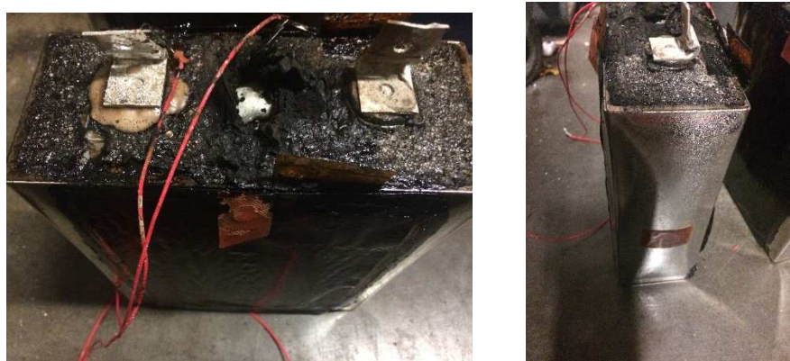
Figure 10 -11 – Photographs of cell after test
