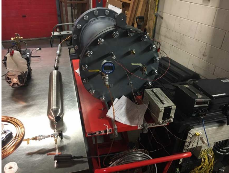
Figure 16 – Battery gas composition test chamber
