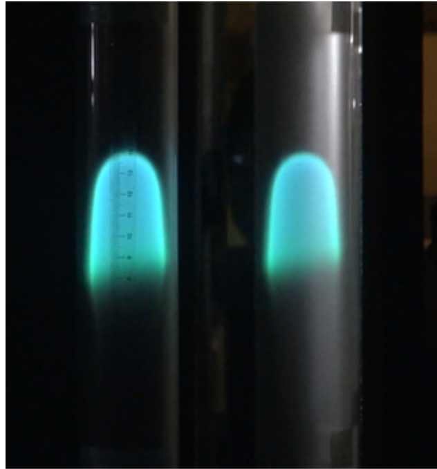
Figure 3. Typical picture of upward flame propagation in 40-mm ID glass tube (flame shape for R32)
